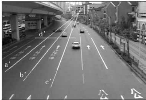
Fig. 2. A snapshot of traffic scenes and the selected calibration target.
