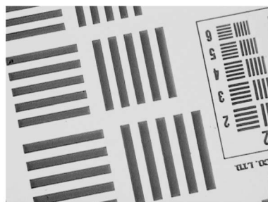
Fig. 1. CCD image of a portion of the Co mask on \text{SiO}_2 surface.
