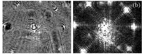
Fig. 3. Experimental results of a 10- \mu m-wide line resolution target. (a) Recorded hologram; (b) amplitude distribution of a four-step phase-shifting hologram.
