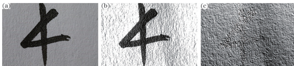
图 9 秀丽笔(先横后竖)笔画的检验效果。(a)显微摄影;(b)镜面反光增强;(c)法线可视化 Fig. 9 Test effect of strokes by Show pen (first horizontal then vertical). (a) Microphotography; (b) mirror reflection enhancement; (c) normal visualization
