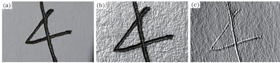
图 7 中性笔(先横后竖)笔画的检验效果。(a)显微摄影;(b)镜面反光增强;(c)法线可视化 Fig. 7 Test effect of strokes by neutral pen (first horizontal then vertical). (a) Microphotography; (b) mirror reflection enhancement; (c) normal visualization
