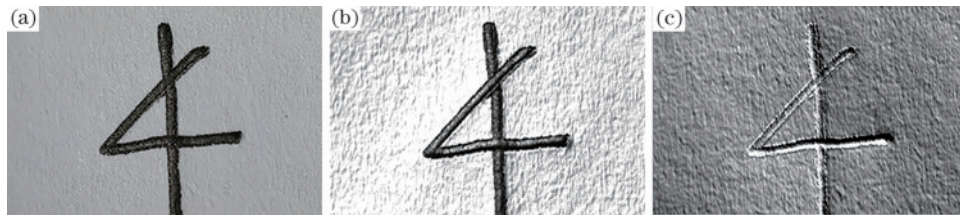
图 8 中性笔(先竖后横)笔画的检验效果。(a)显微摄影;(b)镜面反光增强;(c)法线可视化 Fig. 8 Test effect of strokes by neutral pen (first vertical then horizontal). (a) Microphotography; (b) mirror reflection enhancement; (c) normal visualization
