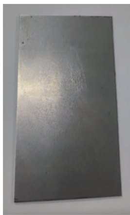
图 9 冷轧钢板待清洗试样 Fig. 9 Sample of cold rolled steel plate to be cleaned
