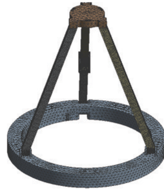
图 7 次镜展开机构的有限元模型 Fig. 7 Finite element model of the secondary unfolded mechanism
