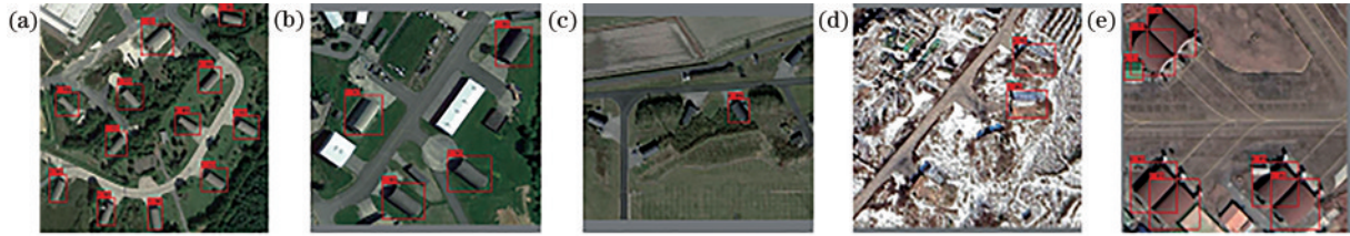
图 13 YOLOv3 检测结果。(a)多目标分布;(b)包含易混淆目标;(c)多方向小目标;(d)雪覆盖下目标;(e)双联飞机掩体 Fig. 13 Results of YOLOv3. (a) Multi-objective distribution; (b) with confusing objectives; (c) multi-directional small objectives; (d) objectives under snow cover; (e) duplex aircraft bunkers
