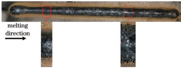
图 12 300 W、5 mm/s 时的涂层形貌及裂纹缺陷 Fig. 12 Coating morphology and cracking defects at 300 W and 5 mm/s
