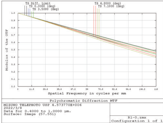
图9 优化后光学系统的MTF Fig. 9 MTF of optimized optical system
