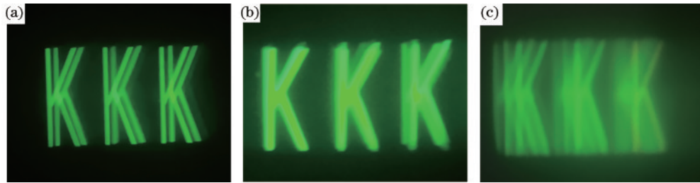
图 18 光栅波导成像测试图。(a)局部光栅周期变化导致重影;(b)光栅波导平整度导致重影;(c)装调误差导致成像模糊重影 Fig. 18 Grating waveguide imaging test chart. (a) Ghosting caused by local grating periodic change; (b) ghosting caused by grating waveguide tilt; (c) imaging blur and ghosting caused by assembly error
