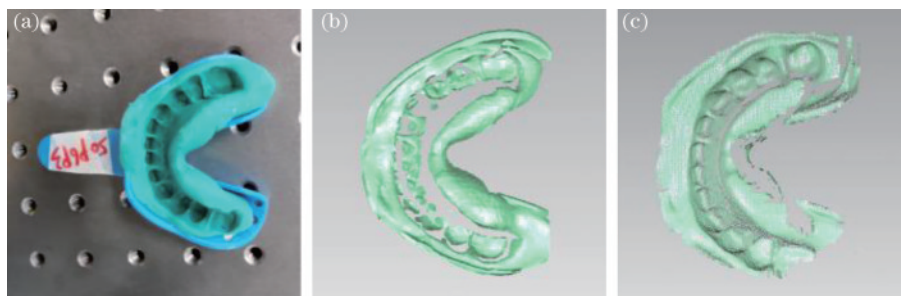
Fig. 7 Experimental scene 2. (a) Measured object of dental impression; (b) result of phase-height mapping method; (c) result of the proposed method
