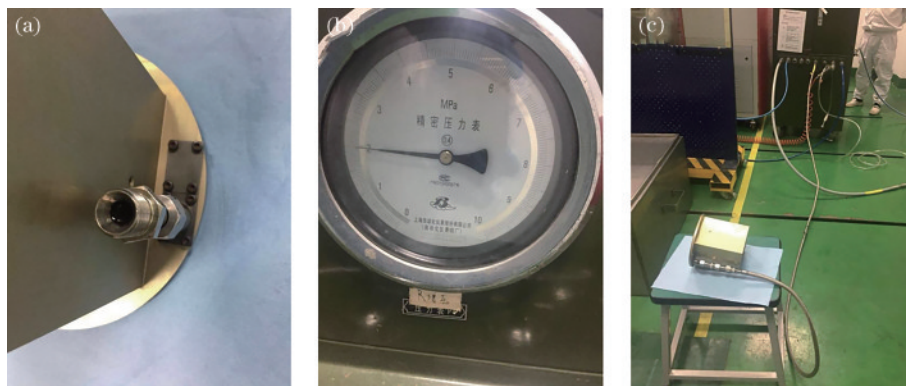
图 14 复杂流道散热元件压力测试。(a)向流道内注水;(b)压力表;(c)压力测试过程 Fig. 14 Pressure test of complex channel cooling element. (a) Filling channels with water; (b) pressure gauge; (c) process of pressure test
