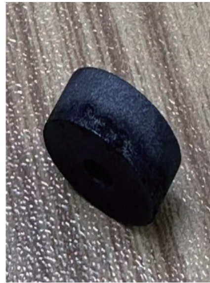
图 10 转盘电极磨损图 Fig. 10 turntable electrode wear diagram
