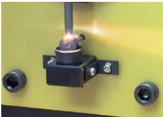
图 8 棒转盘电极装置实验图 Fig. 8 Experimental diagram of rod turntable electrode device
