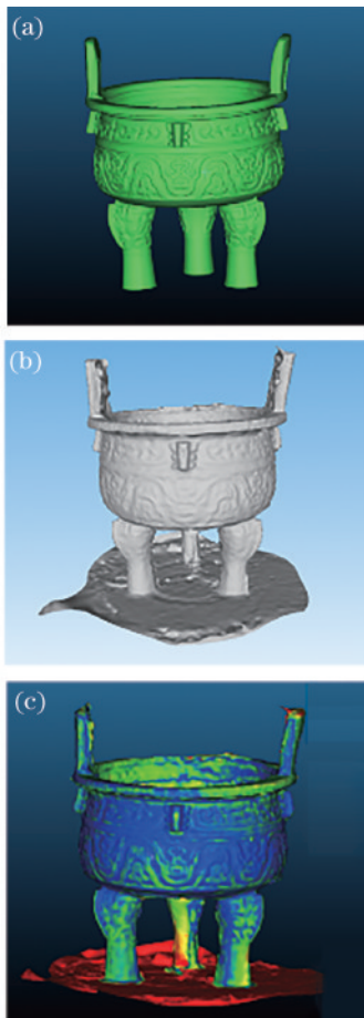
图 13 效果对比。(a)参考模型;(b)所提算法;(c)伪彩色图 Fig. 13 Effect comparison. (a) Reference model; (b) proposed algorithm; (c) pseudo color map
