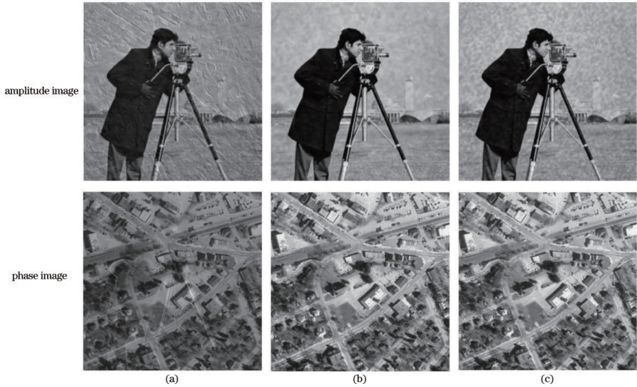
图 3 几种典型的顺序法重建的高分辨率振幅和相位图像。(a)传统 G-S 法;(b) EPRY 法;(c)顺序高斯-牛顿法 Fig. 3 High-resolution amplitude and phase images are reconstructed by several typical sequential methods. (a) Traditional G-S method; (b) EPRY method; (c) sequential Gauss-Newton method
