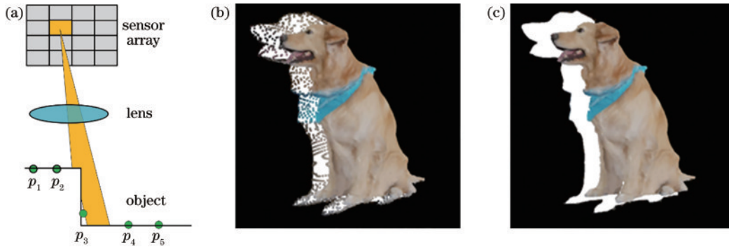
图 6 飞行像素示意图。(a)飞行像素的产生原理;(b)飞行像素引起的误差;(c)去除飞行像素后的效果 Fig. 6 Schematics of flying pixel. (a) Generation principle of flying pixels; (b) errors brought by flying pixels; (c) effect after removing flying pixels
