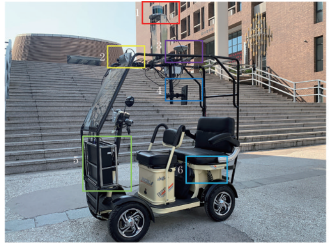
1 — lidar 3 — GPS 5 — industrial PC 2 — camera 4 — car monitor 6 — IMU
