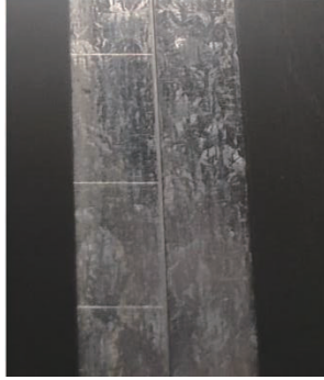
Fig. 2 Weld surface condition and welding fixtures
