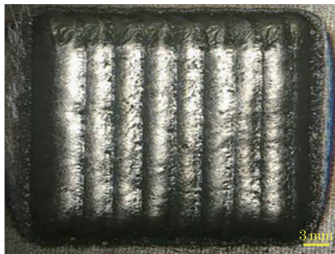
图 2 钴基熔覆涂层的宏观表面形貌 Fig. 2 Macroscopic surface morphology of Co-based cladding layer
