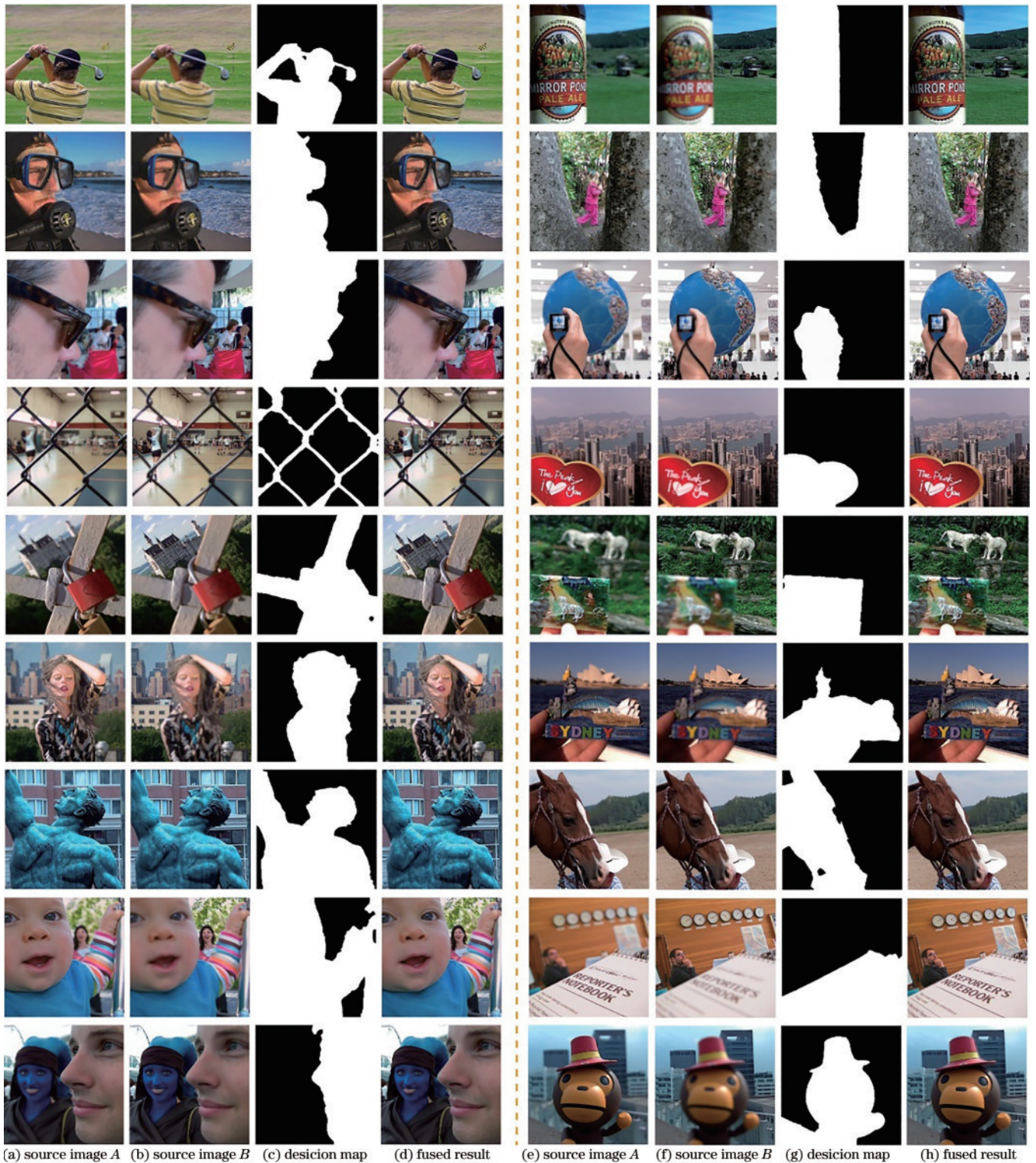
图 6 提出方法更多结果展示。第 1 列到第 4 列, 第 5 列到第 8 列分别展示了 18 幅多聚焦图像融合结果 Fig. 6 More results of proposed method. The first to fourth and fifth to eighth columns show fusion results of 18 pairs of multi-focus images, respectively
