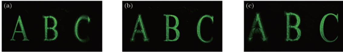
图 4 3D 物体的大尺寸全息显示结果。(a)“A”聚焦时的全息显示结果;(b)“B”聚焦时的全息显示结果;(c)“C”聚焦时的全息显示结果 Fig. 4 Large size holographic display results of 3D scene. (a) Holographic display result when “A” is focused; (b) holographic display result when “B” is focused; (c) holographic display result when “C” is focused
