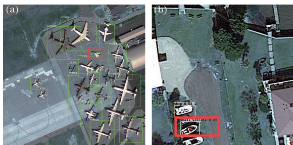
图7 漏检和错检示例。(a)漏检;(b)错检 Fig. 7 Examples of miss detection and error detection. (a) Miss detection; (b) error detection
