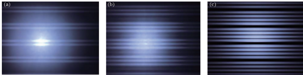
图 5 不同曝光度下的 LED-ID 光条纹码的效果。(a) 1/500; (b) 1/1000; (c) 1/2000 Fig. 5 Effects of LED-ID light stripe code under different exposure. (a) 1/500; (b) 1/1000; (c) 1/2000
