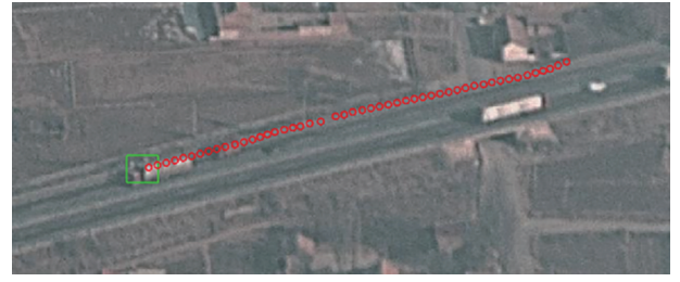
图 1 根据单应变换将目标历史位置映射到当前参考帧的结果 Fig. 1 Result of mapping the historical position of the target to the current reference frame according to homography transformation
