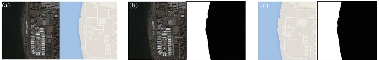
图 5 实验数据。(a)原始数据集;(b)本文使用的数据集;(c)通过海陆二值化操作将谷歌地图转换成海陆二值化图像 Fig. 5 Experimental data. (a) Original dataset; (b) dataset used in this paper; (c) Google Maps converted into sea-land binarized image by sea-land binarization operation
