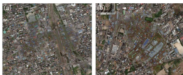
图 2 对数变换自适应 \gamma 补偿方法对不同影像的补偿效果 Fig. 2 Compensation effects of logarithmic transformation adaptive \gamma compensation method for different images
