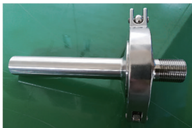
图 7 调频连续波光纤维压力传感器的传感头结构实物 Fig. 7 Structure of sensing head of frequency modulated continuous wave fiber optic pressure sensor
