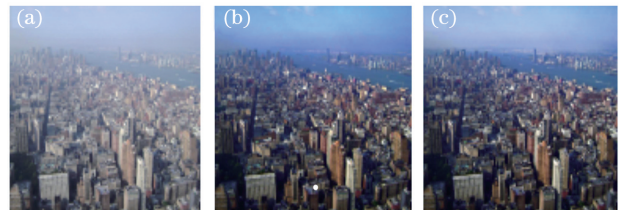
图 5 明亮区域的复原效果。(a)有雾图像;(b)修正前的去雾图像;(c)自适应修正后的去雾图像 Fig. 5 Restoration effect of bright area. (a) Hazy image; (b) dehazing image before correction; (c) dehazing image after adaptive correction
