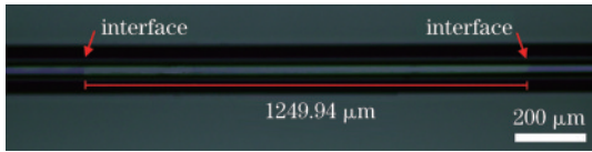
图 7 扫描长度为 1.5 mm, HEAT 为 500 时的光纤侧视图 Fig. 7 Later view of the treated fiber at scanning length of 1.5 mm and HEAT of 500
