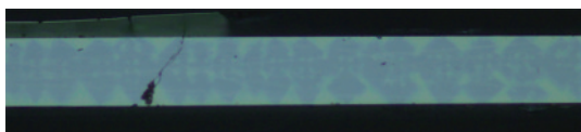
图 4 扫描长度为 8 mm, HEAT 为 700 时的纤芯侧剖面 Fig. 4 Profile section of the treated fiber at scanning length of 8 mm and HEAT of 700
