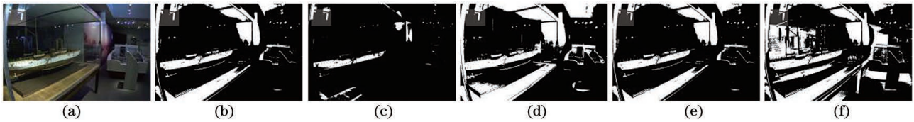
图 4 算法分割结果。(a)原始图像 1;(b)Otsu;(c)二维最大熵;(d)文献[18]中算法;(e)文献[23]中算法;(f)本文算法 Fig. 4 Algorithm segmentation results. (a) Original image 1; (b) Otsu; (c) 2D maximum entropy; (d) algorithm in Ref. [18]; (e) algorithm in Ref. [23]; (f) proposed method
