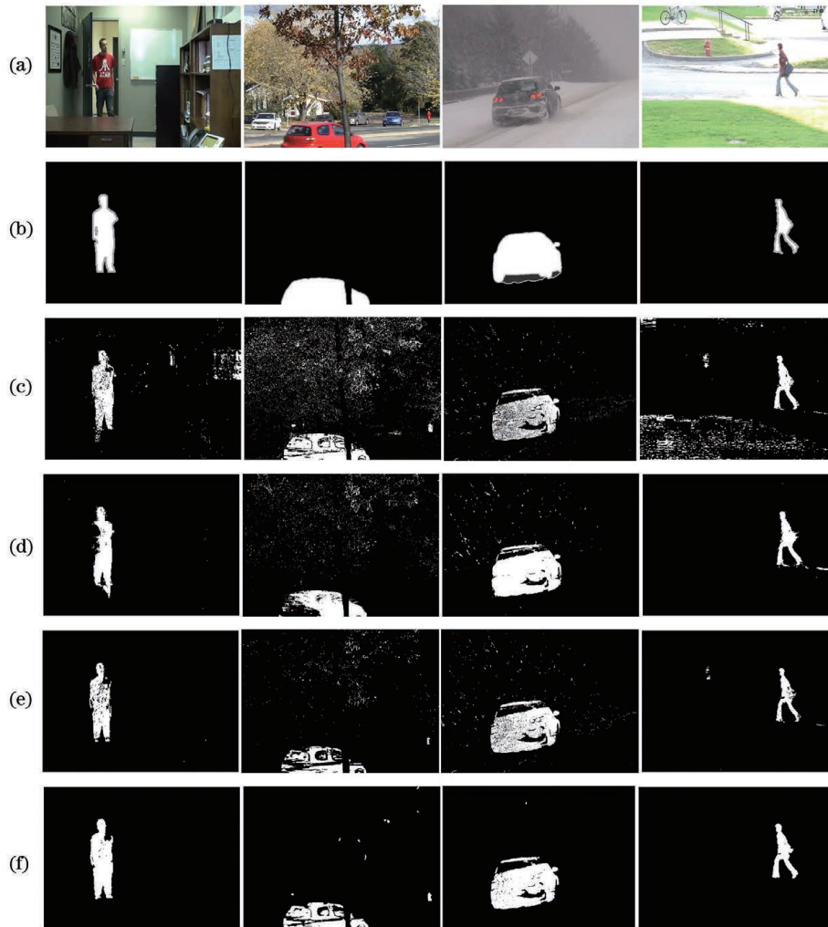
图 5 运动目标的检测结果。(a)视频帧;(b)真值图;(c)ViBe 算法;(d)高斯混合模型;(e)文献[22];(f)所提算法 Fig. 5 Detection results of moving object. (a) Video frames; (b) ground truth; (c) ViBe algorithm; (d) Gaussian mixture model; (e) Ref. [22]; (f) proposed algorithm
