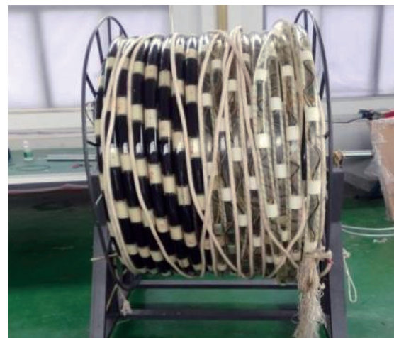
图 11 拖曳线列阵 FOH 的实物图 [102] Fig. 11 Physical picture of the towed line array FOH [102]
