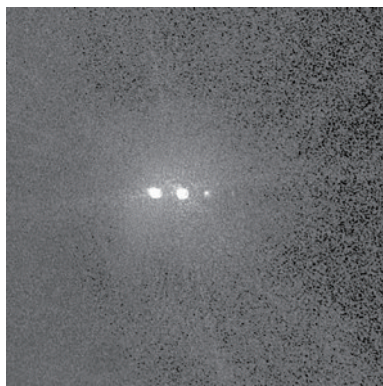
图 3 直径为 10 \mu\text{m} 的麻点散射场分布 Fig. 3 Scattering field distribution of the pit with diameter of 10 \mu\text{m}
