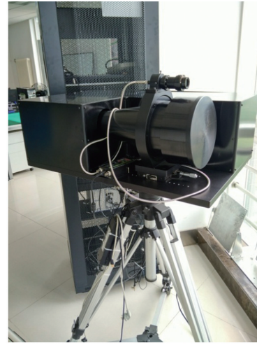
Fig. 1 Experimental setup of the computational ghost imaging system
