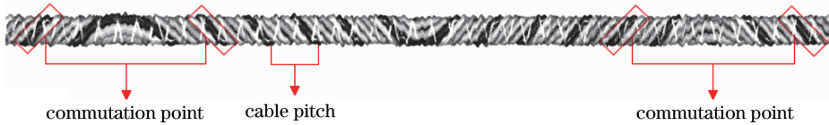
图 3 换向点与节距 Fig. 3 Commutation point and cable pitch
