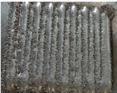
图1 能量密度小于等于 19 \text{ J} \cdot \text{mm}^{-2} 时的316L涂层表面 Fig. 1 Surface of 316L coating when energy density is less than or equal to 19 \text{ J} \cdot \text{mm}^{-2}
