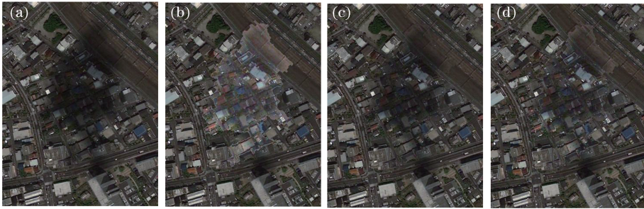
图3 三种方法得到的补偿结果。(a)原始影像;(b)对数变换结果;(c)局部补偿结果;(d)联合补偿结果 Fig. 3 Compensation results from three methods. (a) Original image; (b) logarithmic transformation result; (c) local compensation result; (d) joint compensation result
