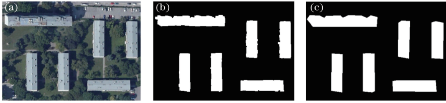
图 4 建筑物边缘轮廓初步拟合效果。(a)原始遥感影像;(b)初始提取的建筑物结果;(c)初步拟合后的建筑物轮廓 Fig. 4 Preliminary fitting effect of building edge contour. (a) Original remote sensing image; (b) initial results of building extraction; (c) building contour after preliminary fitting
