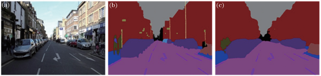
图5 基于 Cityscapes 数据集本文分割算法的示例结果图。(a)原始图片;(b)真实分割结果;(c)本文算法分割结果 Fig. 5 Example results of proposed segmentation algorithm based on Cityscapes dataset. (a) Original image; (b) true segmentation result; (c) result of proposed algorithm
