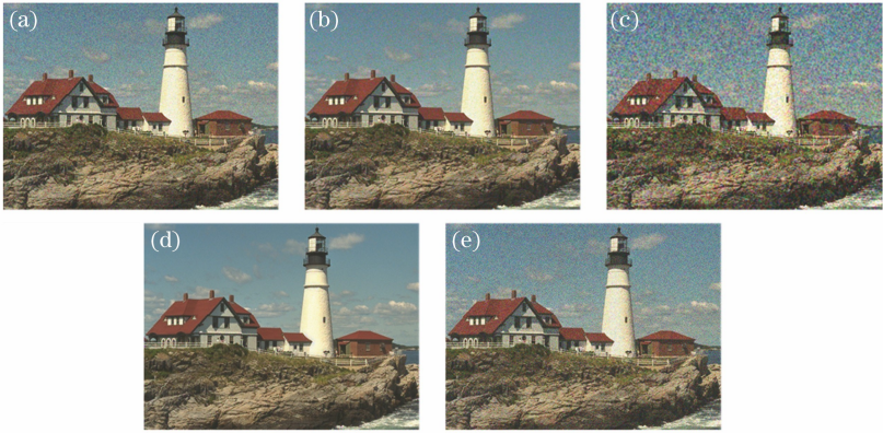
图 1 5 幅不同失真类型的图像。(a) 加性高斯噪声; (b) 色彩分量上的加性噪声; (c) 空间相关噪声; (d) 掩蔽噪声; (e) 高频噪声 Fig. 1 Five images of different distortion types. (a) Additive Gaussian noise; (b) additive noise in color component; (c) spatially correlated noise; (d) masked noise; (e) high frequency noise
