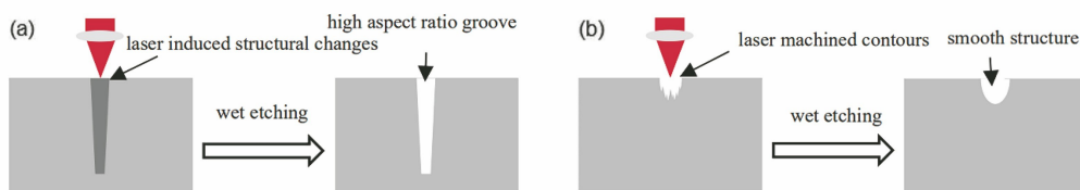
图 1 飞秒激光辐照结合湿法腐蚀加工实验流程。(a)飞秒激光结合湿法腐蚀制备高纵横比狭槽; (b)飞秒激光结合湿法腐蚀制备微透镜
