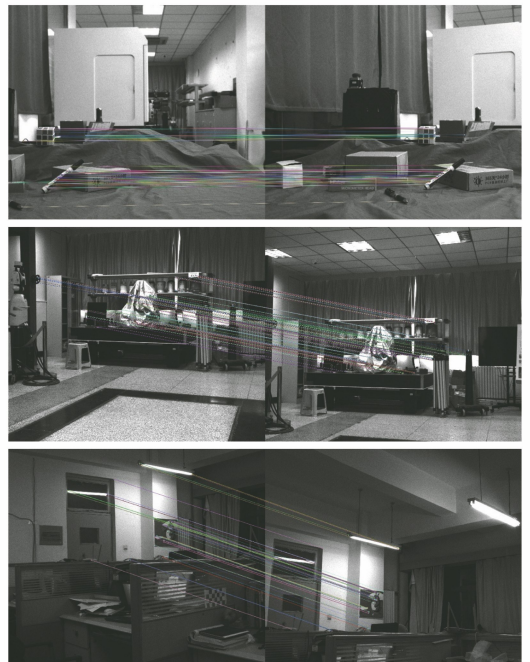
图 11 三组图像采用 RANSAC 剔除外点后的匹配结果 Fig. 11 Match results of three sets of images after removing outliers by RANSAC
