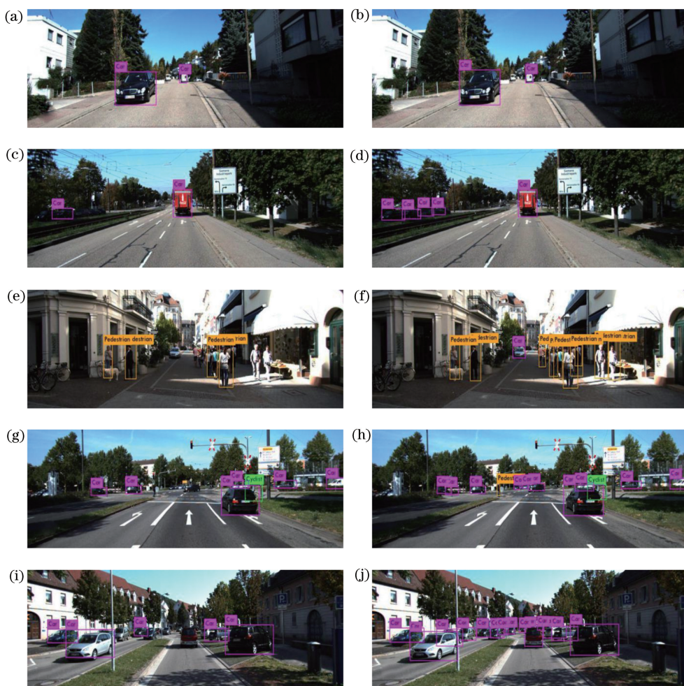
图9 检测结果图。(a)(c)(e)(g)(i) YOLOv2 模型检测结果;(b)(d)(f)(h)(j) RF-YOLOv2 模型检测结果 Fig. 9 Detection results. (a)(c)(e)(g)(i) Detection results of YOLOv2 model; (b)(d)(f)(h)(j) detection results of RF-YOLOv2 model
