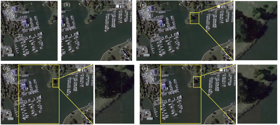
图 13 Harbor 图像在三种融合策略下的对比。(a)(b)原图;(c) S型融合;(d)直接平均融合;(e)渐入渐出融合 Fig. 13 Comparison of three fusion strategies for images of harbor. (a)(b) Original images; (c) S-type fusion; (d) direct average fusion; (e) gradual integration
