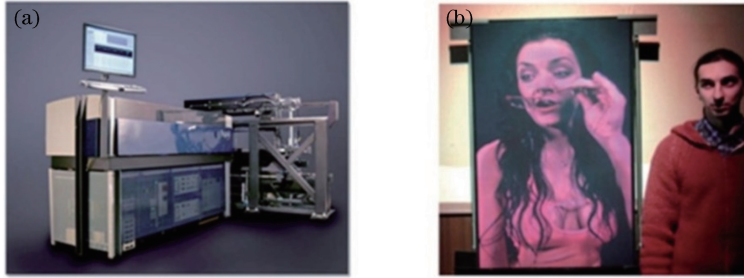
图4 Geola的全息体视图打印系统。(a) Geola的脉冲激光打印系统;(b)该系统制作的高质量大幅面全彩色全息体视图 Fig. 4 Holographic stereogram printing system designed by Geola. (a) Pulse laser printing system of Geola; (b) full color holographic stereogram with high quality and large format made by this system
