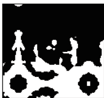
图 9 图 5(c)的基本全局阈值法和大津法分割结果 Fig. 9 Segmentation results of Fig. 5(c) using basic global threshold method and Otsu method
