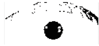
图 3 取灰度均值最小值为阈值进行二值处理 Fig. 3 Take the minimum mean grayscale value as threshold value for binary processing
