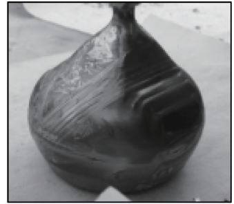
图 4 有保温罩下 B_2O_3 作为液封剂时生长的 GaSb 夹晶 Fig. 4 GaSb clip crystal grown by B_2O_3 as liquid sealing agent with thermal insulation cover
