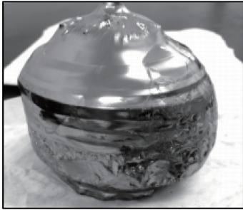
图 3 无保温罩下 B_2O_3 作为液封剂时生长的 GaSb 多晶 Fig. 3 GaSb polycrystal grown by B_2O_3 as liquid sealing agent without thermal insulation cover
