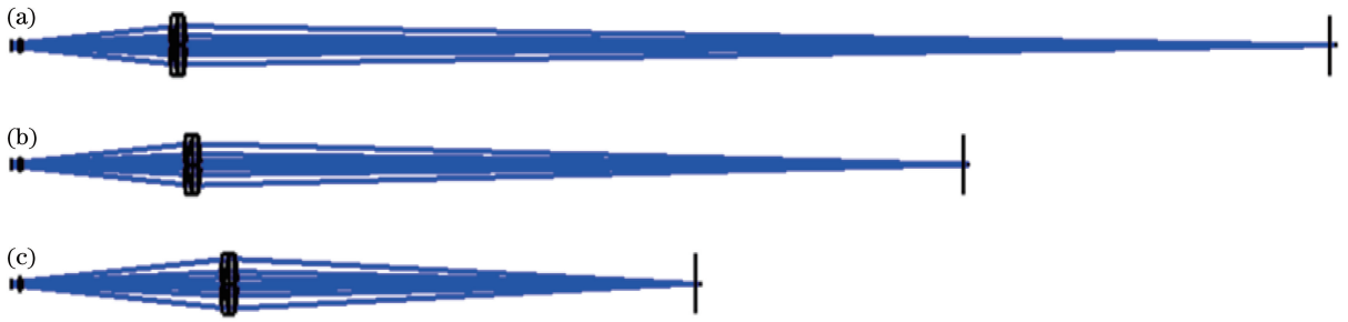
图2 不同聚焦距离下的聚焦图。(a)聚焦距离为 300 mm;(b)聚焦距离为 500 mm;(c)聚焦距离为 750 mm Fig. 2 Focus figures under different focusing distances. (a) Focusing distance is 300 mm; (b) focusing distance is 500 mm; (c) focusing distance is 750 mm
