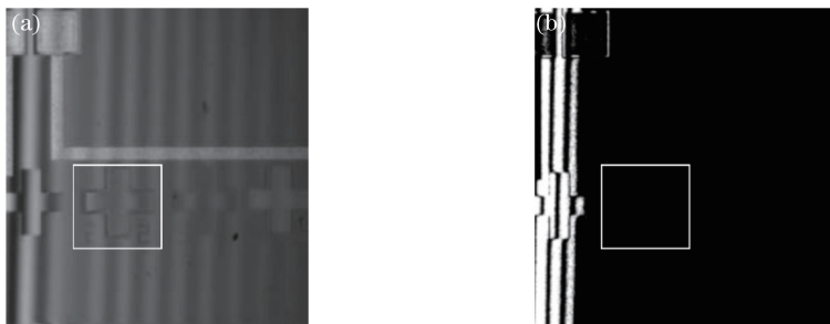
图 8 扫描下限的确定。(a)扫描下限处的 CCD 图像;(b) ViBe 算法分割并二值化处理后的扫描下限处图像 Fig. 8 Determination of scanning lower limit. (a) CCD image at scanning lower limit position; (b) image at scanning lower limit position after ViBe extraction and binaryzation treatment
