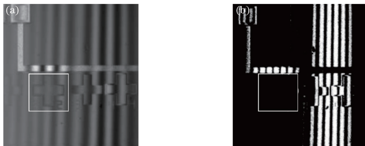
图 7 扫描上限的确定。(a)扫描上限处的 CCD 图像;(b) ViBe 算法分割并二值化处理后的扫描上限处图像 Fig. 7 Determination of scanning upper limit. (a) CCD image at scanning upper limit position; (b) image at scanning upper limit position after ViBe extraction and binaryzation treatment
